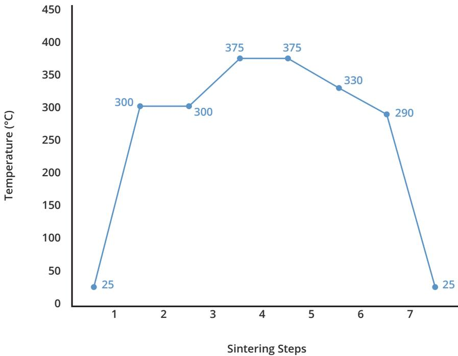
Table 3-Typical sintering cycle for INOFLON® Fine cut granular PTFE, Solid billets:
