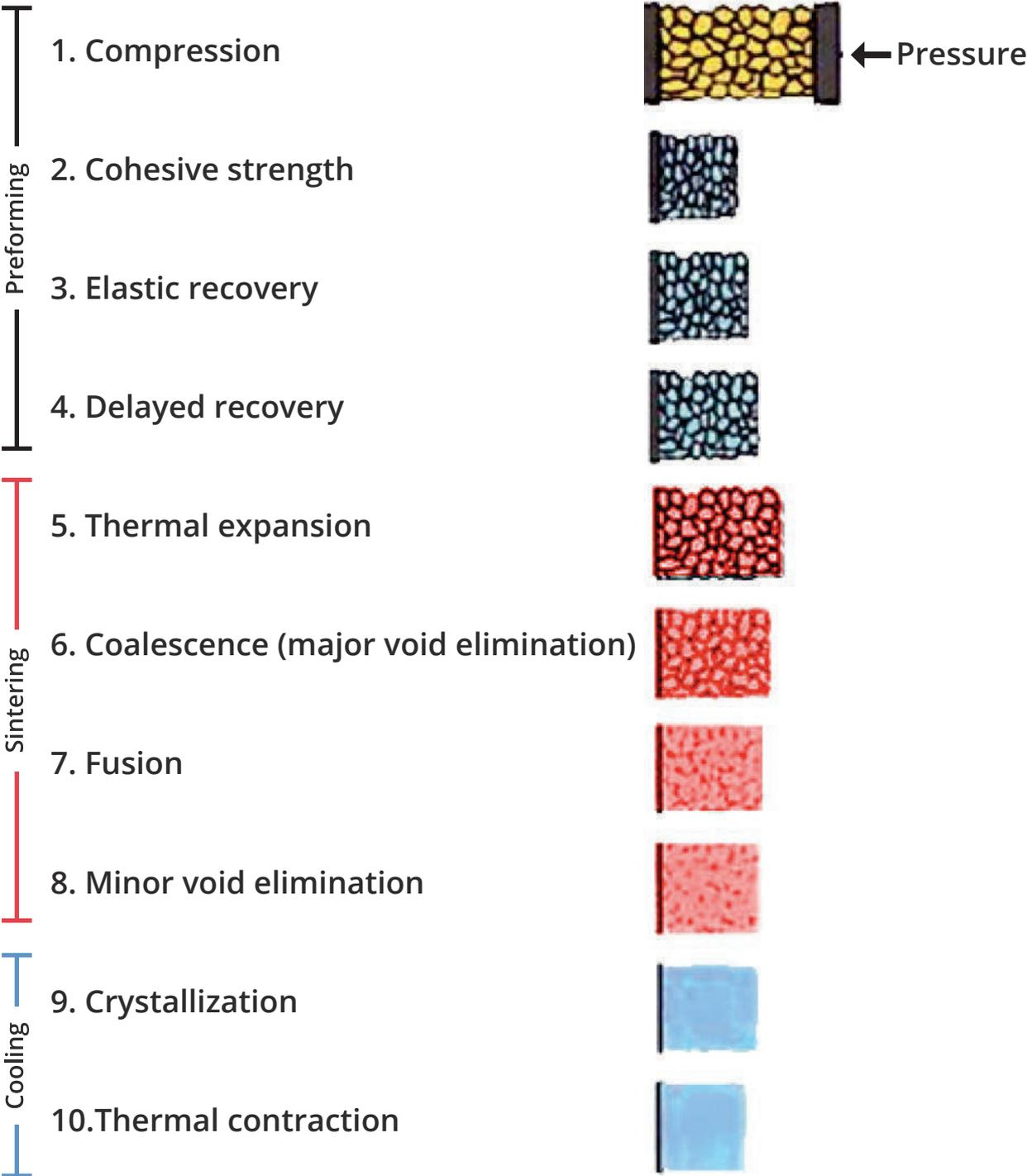
Figure 1- Schematic diagram of preforming and sintering sequence with PTFE
