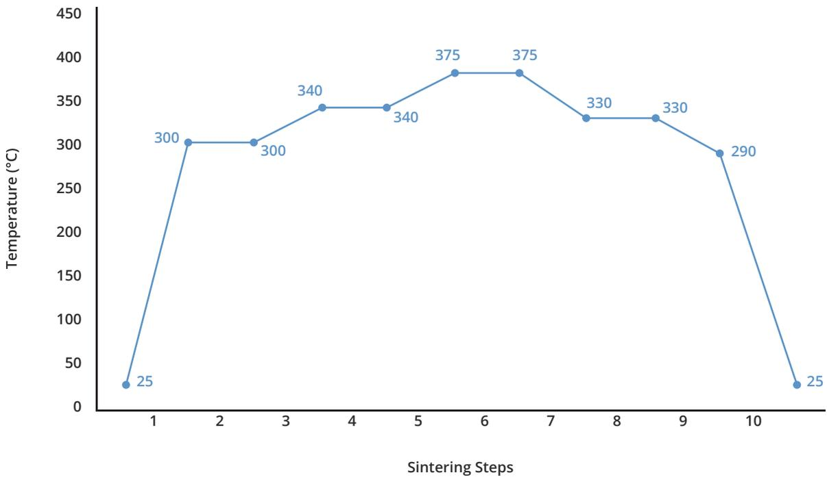
Table 4 -Typical sintering cycle for INOFLON® Fine cut granular PTFE, Annular billets:
